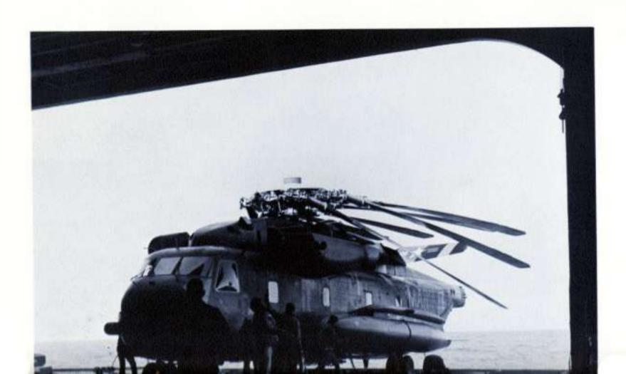
From a stowed configuration, the aircraft can be spread and ready for flight checkout in less than two minutes. Primary flight systems also can be checked in the stowed position.
