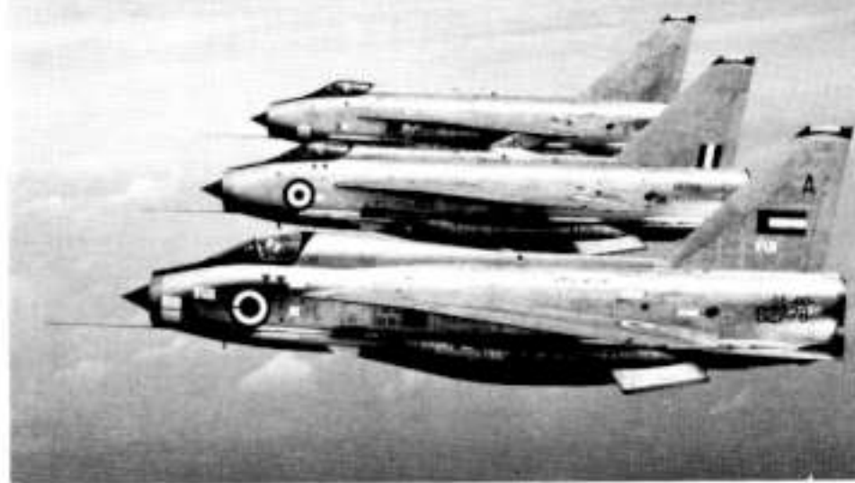
An excellent study of the two-seat T.55 for Kuwait (with Firestreaks), an F.6 of the RAF (with Red Tops) and an F.53 for Saudi Arabia (guns and 1,000lb bombs)
