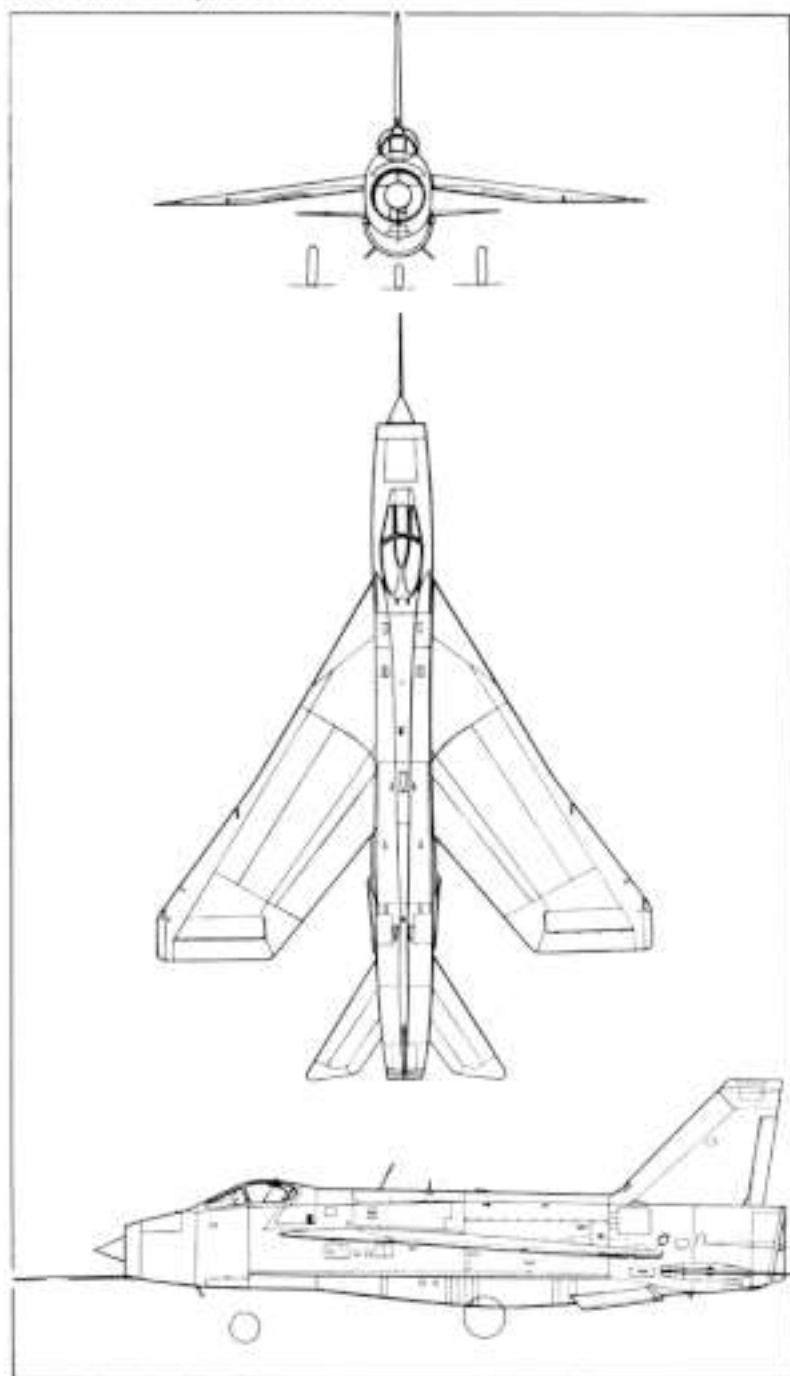
Left, general-arrangement drawing of the Lightning F.53. Right, the aircraft as it appears with a few of the many combinations of stores which may be carried
