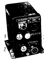
Fig. 142. Marker Receiver MПП-48П 1 - circuit I tuner; 2 - circuit II tuner; 3 - jack for plug of check instrument for measuring relay current.
