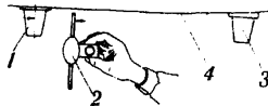
Fig. 157. Checking Radiation Power of Radio Range Finder 1 - transmitting antenna CD-1; 2 - power-level indicator; 3 - receiving antenna; 4 - aircraft skin.
