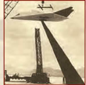
Above: The Northrop XST going on the pole for RCS testing.
