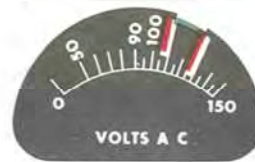
VOLTMETER (AC GENERATORS AND INVERTERS)
