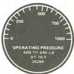
FIRE EXTINGUISHER SYSTEM PRESSURE GAGE
