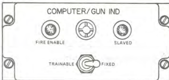
M COMPUTER/GUN INDICATOR CONTROL PANEL
