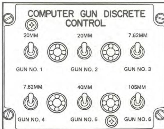
G COMPUTER GUN DISCRETE CONTROL PANEL
