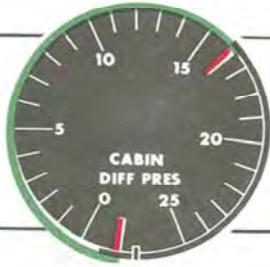
CABIN DIFFERENTIAL PRESSURE GAGE
