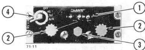
E TACAN CONTROL PANEL 1. CHANNEL INDICATOR 2. CHANNEL SELECT KNOBS 3. VOLUME CONTROL 4. FUNCTION SELECT KNOB
