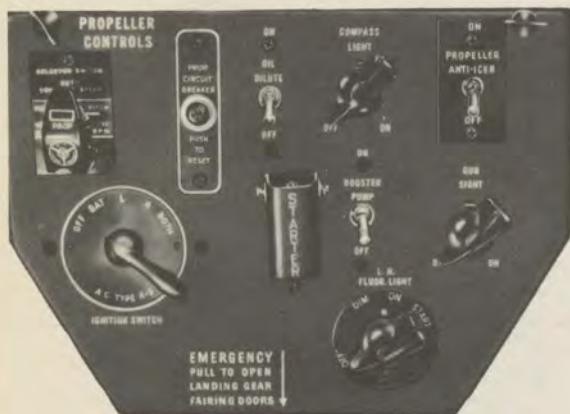
Fig. 31 PILOT'S SWITCH PANEL
