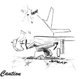
Handgrip on fuselage side must not be used for a step, as it may break and cause injury.
