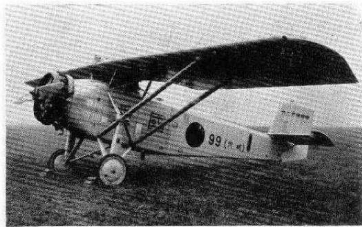
1932. Army 92 Reconnaissance. All the World's Aircraft 420 h.p. Mitsubishi-built Jaguar motor. Span—41 ft. 8 ins. Top speed—136 m.p.h. One-time standard Army reconnaissance type.
