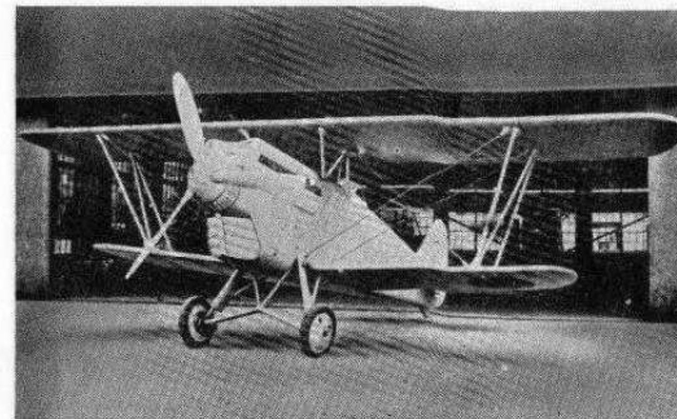
1935. Army 95 Fighter. 600 h.p. Kawasaki-built B.M.W. motor. Span—33 ft. 0 in. Top speed—250 m.p.h. One version had spatted undercarriage.
