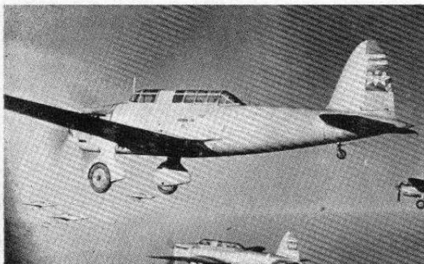
1938. Army 98 Reconnaissance-bomber. MARY 900 h.p. Kawasaki Type 98 motor. Span—47 ft. 7 ins. Top speed—236 m.p.h. Used in China as standard bomber.
