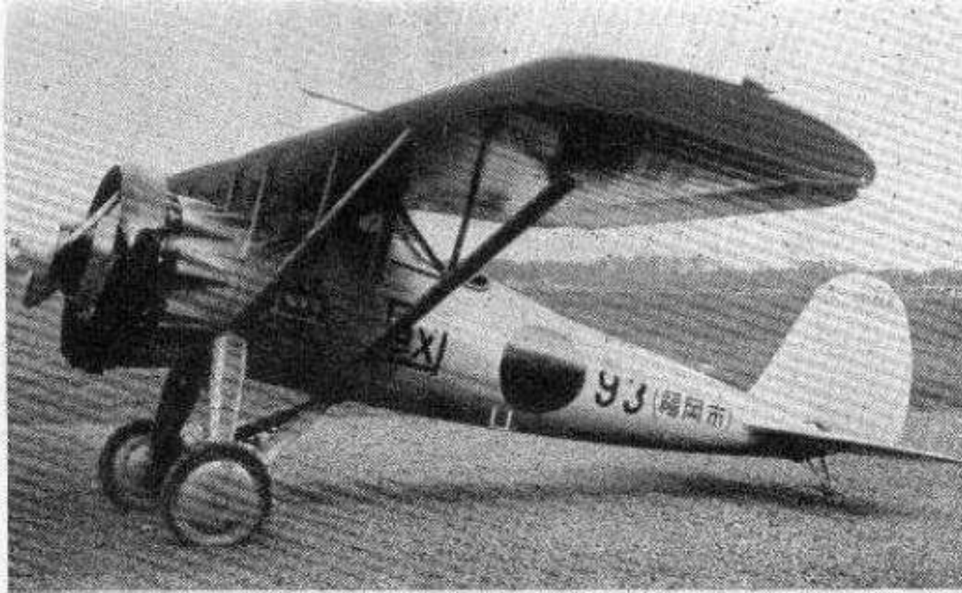
1931. Army 91 Fighter. 450 h.p. Nakajima-built Jupiter motor. Span—36 ft. 0 in. Top speed—201 m.p.h. One-time standard Army type.
