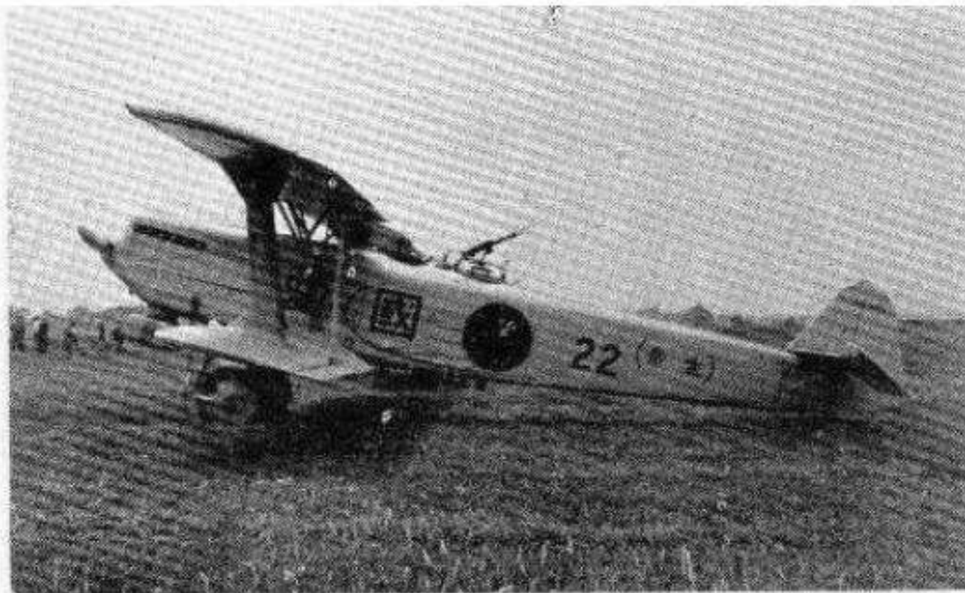
1928. Army 88 Reconnaissance. 450 h.p. Kawasaki-built B.M.W. motor. Span—49 ft. 10 ins. Top speed—136-142 m.p.h. One-time standard Army type.
