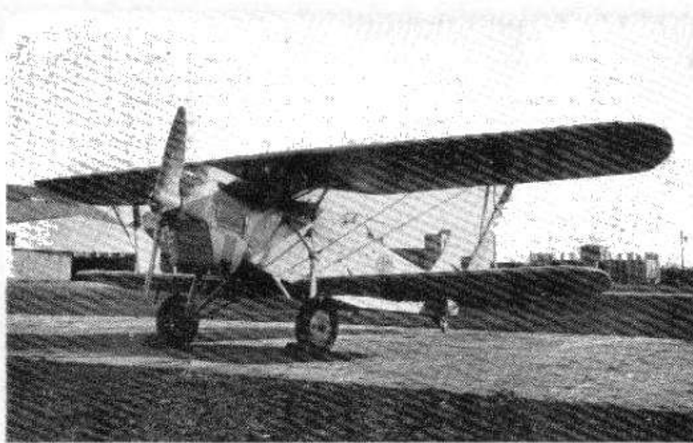
1933. Army 93 Light Bomber. 600 h.p. Kawasaki-built B.M.W. motor. Span—42 ft. 8 ins. Top speed—161 m.p.h. Used in quantity in China.
