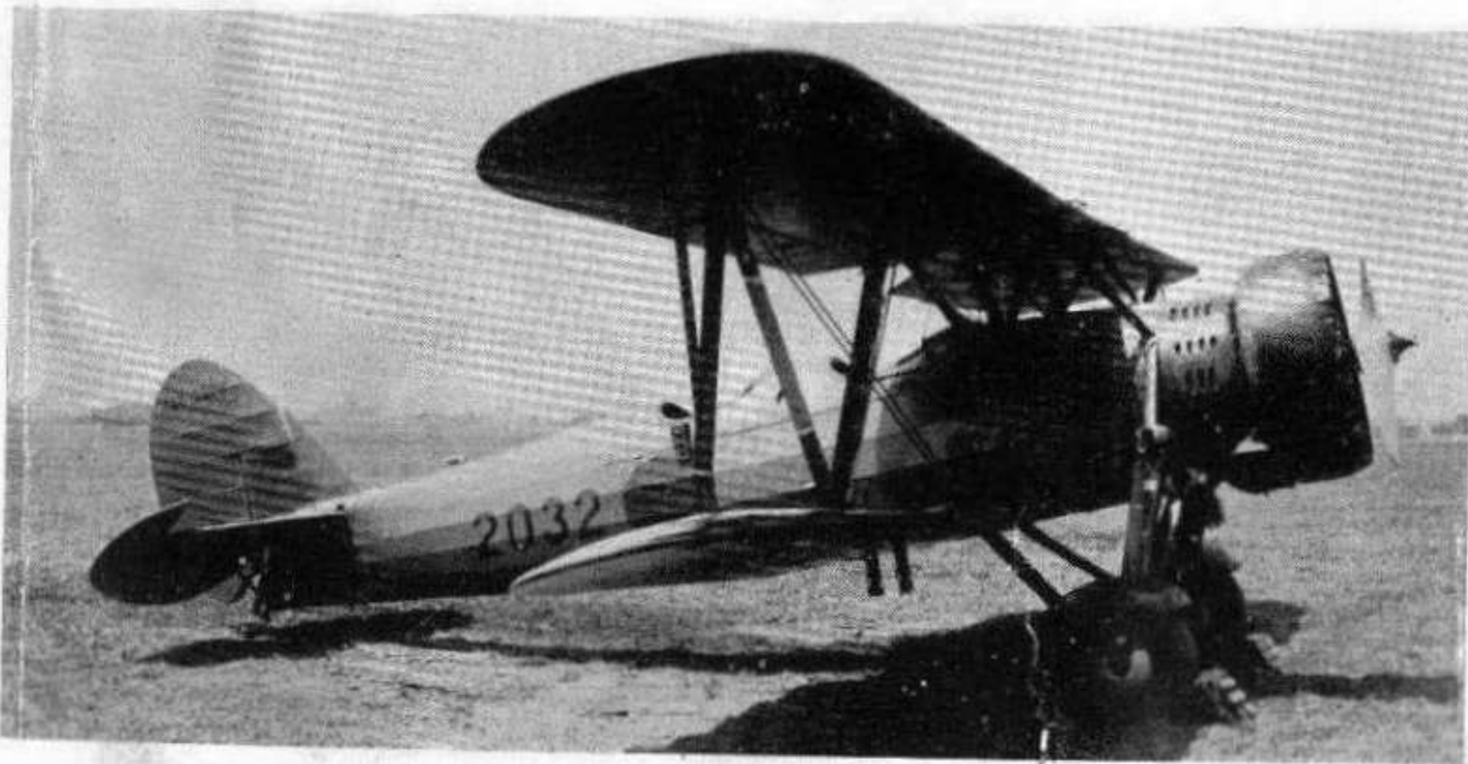
TATIKAWA ARMY 95-1. Built by the Tatikawa Aircraft Co. (until 1936 the Ishikawajima Aircraft Co., Ltd.). This type is one of the few known Japanese advanced trainers. One 350 h.p. Type 95 motor. Span : 32 ft. 9 in. Top speed : 142 m.p.h.
