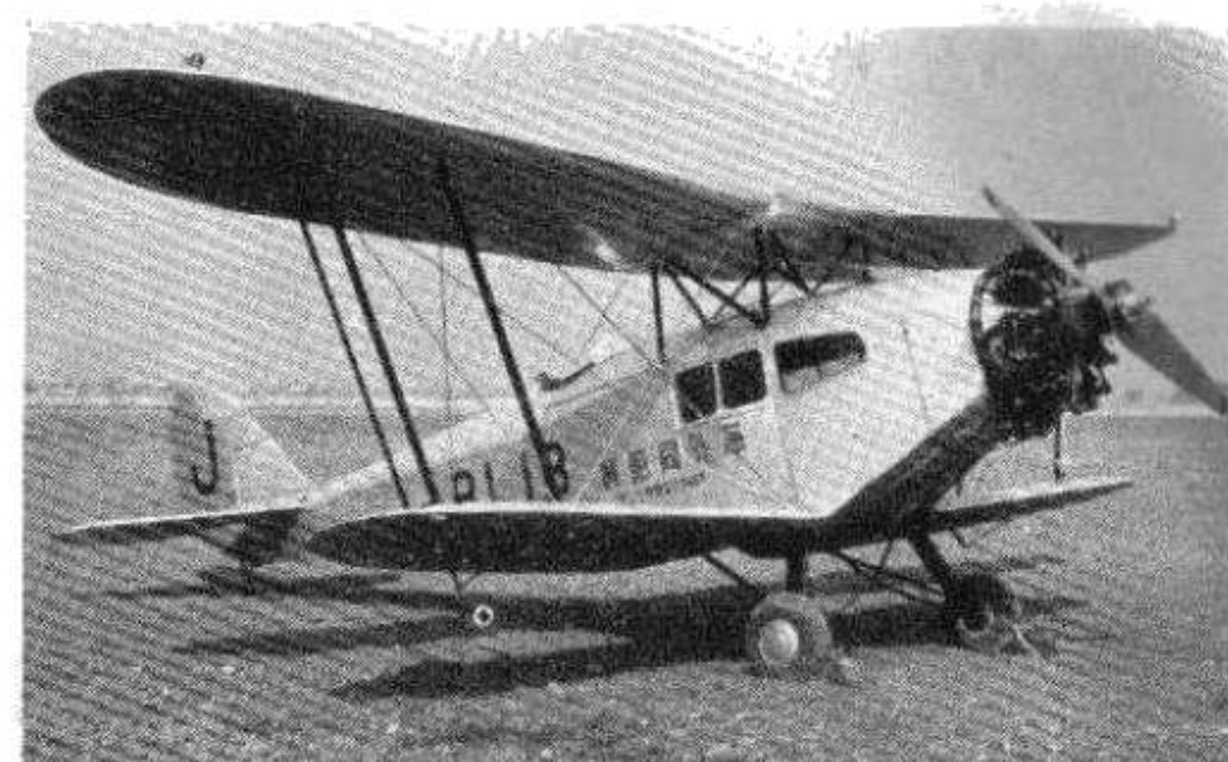
1935. KR.2 Light Transport. 130 h.p. T.G.D. Jimpu motor. Span—30 ft. 2 ins. Top speed—130 m.p.h. One version has covered cockpit.
