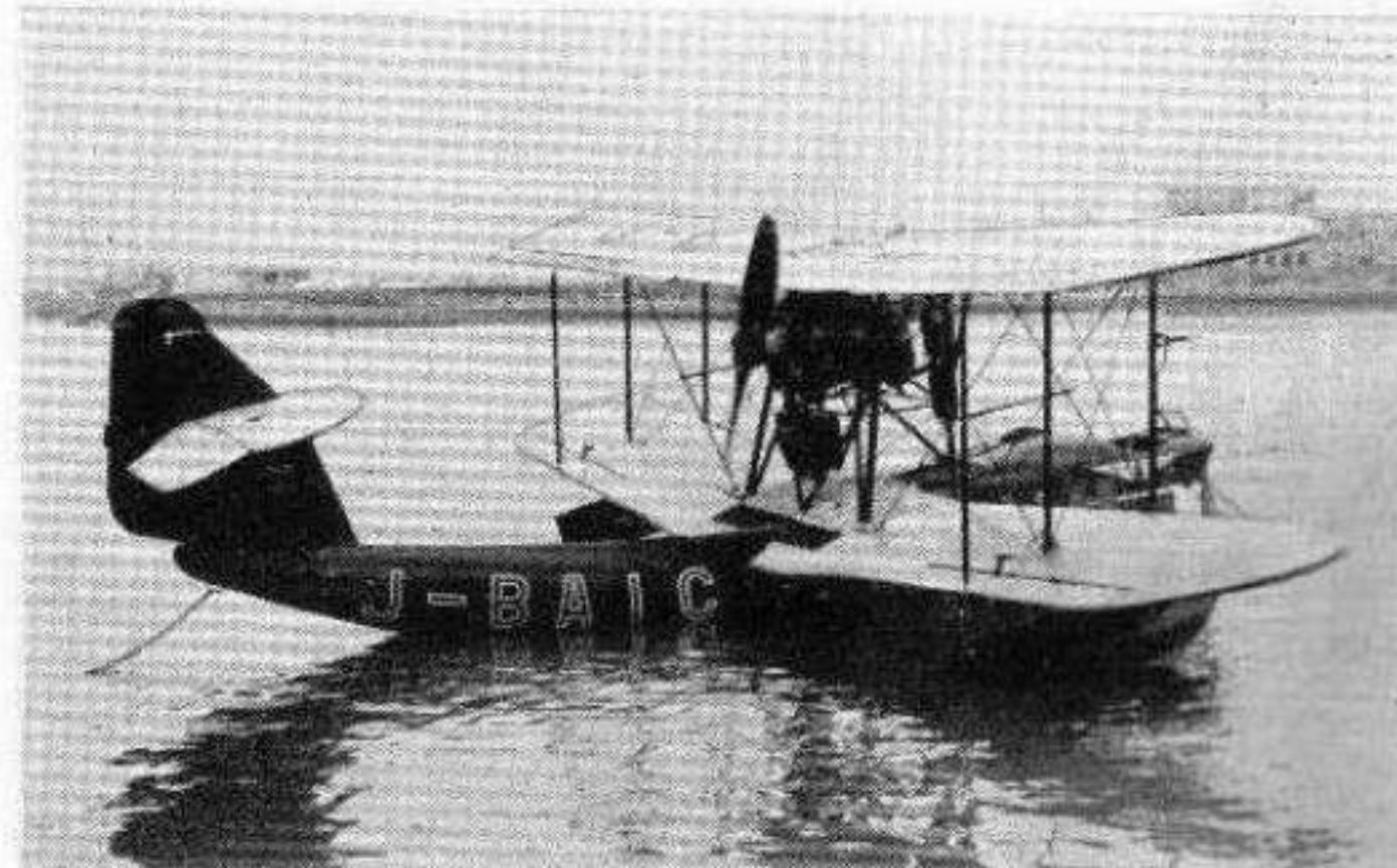
1934. AB-4B Six-passenger flying-boat. 450 h.p. Napier Lion pusher motor. Span—45 ft. 11 ins. Top speed—96 m.p.h. Earlier AB4—has 300 h.p. T.G.D. motor.
