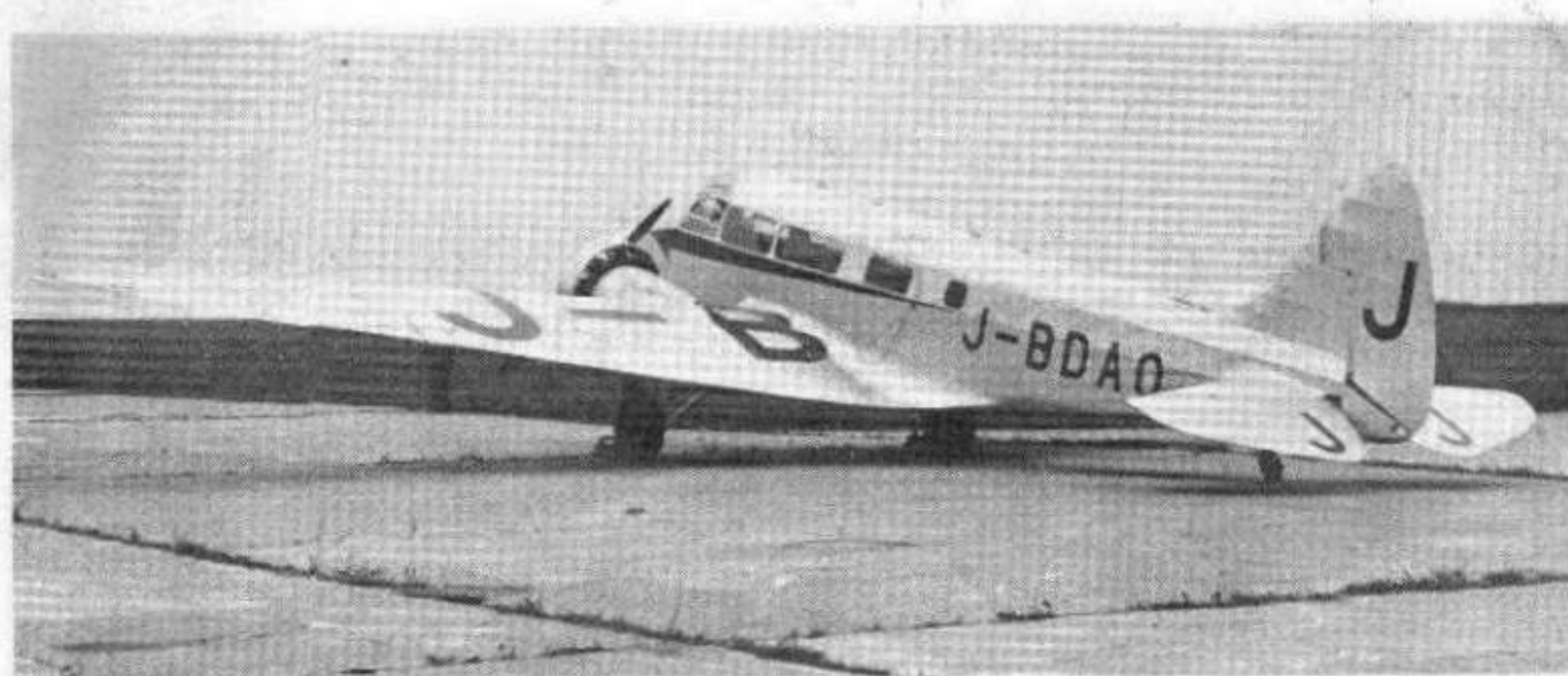
MITSUBISHI HINAZURU (Young Crane). This aeroplane is the British Airspeed Envoy built under licence by the Mitsubishi Company. It is in service in small numbers with the Japan Airways Co., Ltd. Two 240 h.p. Mitsubishi-built Armstrong Siddeley Lynx IVc motors. Span : 52 ft. 4 ins. Top speed 174 m.p.h. Accommodation : 1 pilot and 8 passengers.
