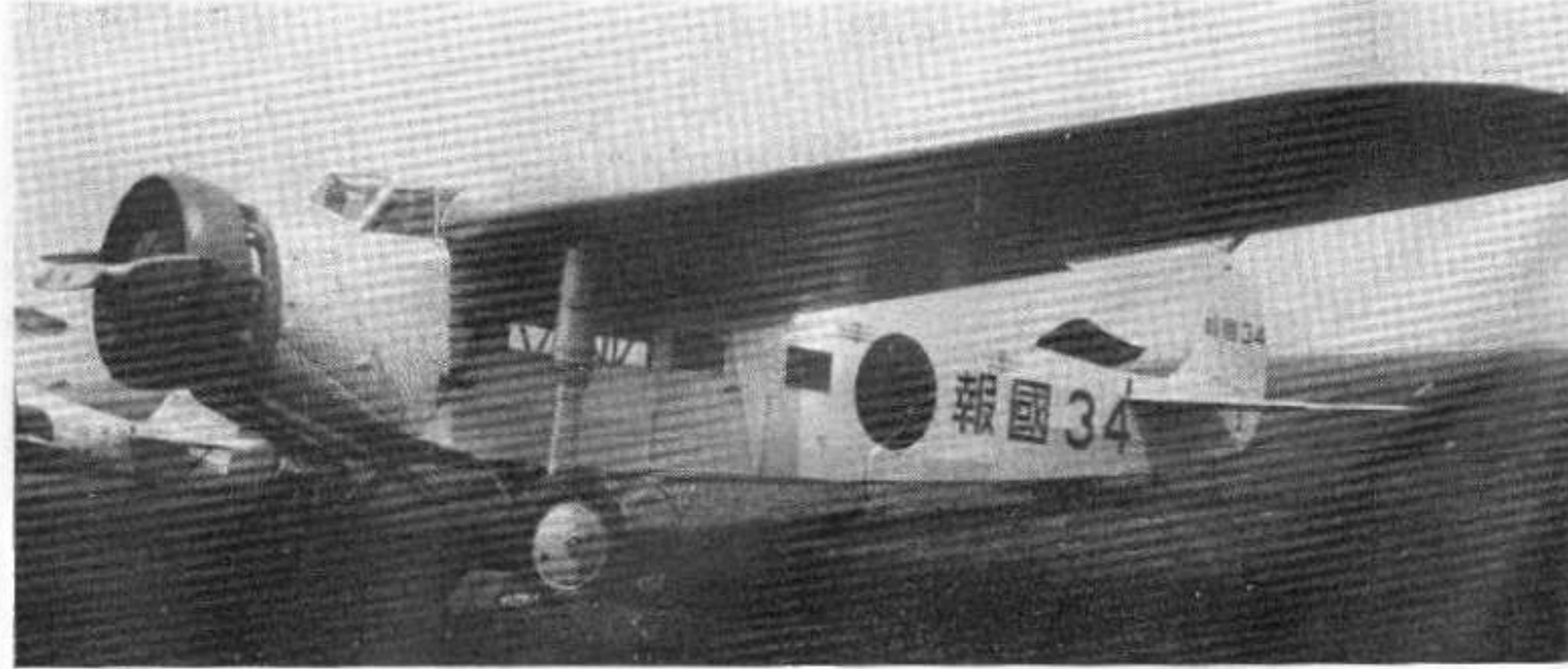
NAKAJIMA-FOKKER UNIVERSAL . Built under licence, this American Fokker design is still in service with the Japan Airways Company and the Japanese Army and Navy Air Services. One 450 h.p. Nakajima-built Jupiter motor. Span : 50 ft. 8 ins. Top speed : 142 m.p.h. Accommodation : 2 crew and 6 passengers.
