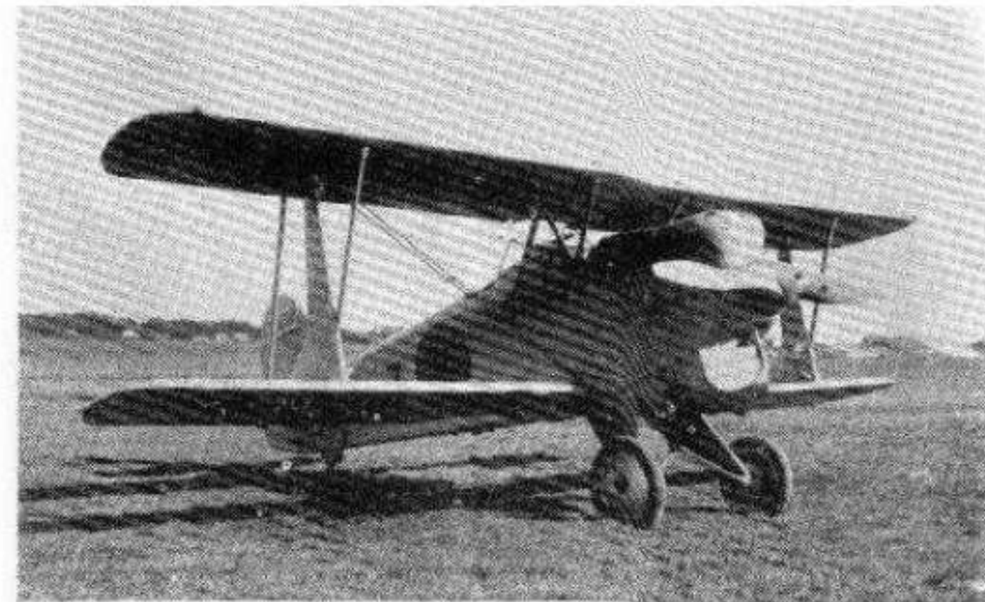
1932. Army 92 Fighter. 450 h.p. Kawasaki-built B.M.W. motor. Span—31 ft. 2 ins. Top speed—205 m.p.h. One-time standard Army type.
