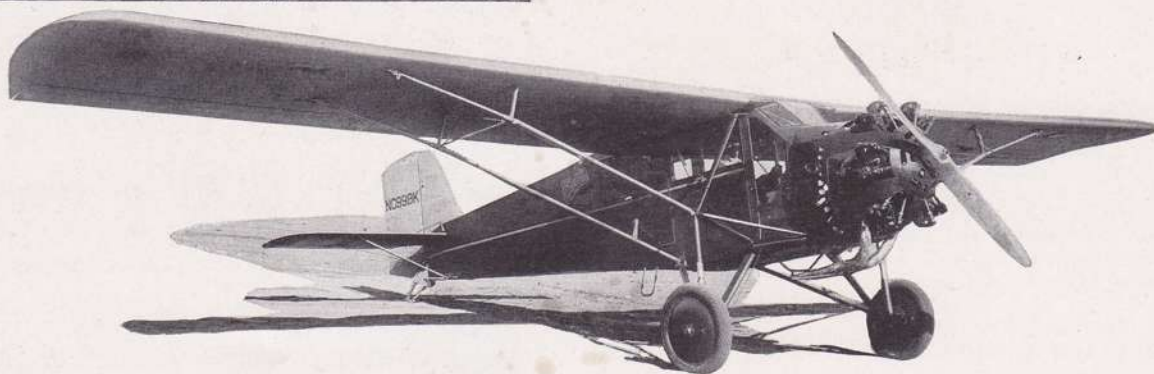
Above. The Curtiss Robin, first private airplane ever built on mass production lines patterned after those found at that time in the automobile factories of the nation.
