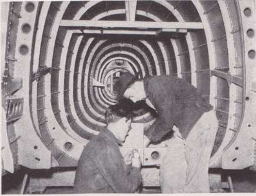
Bulkheads and Stringers—The Belly of the AT-9.
