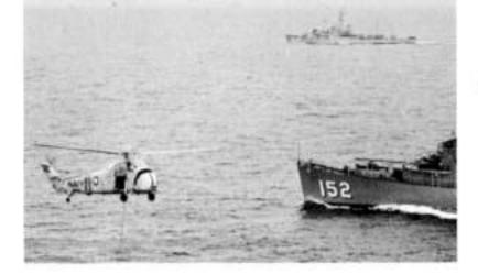
SH-34J. This sonar-equipped, Sikorsky S-58 helicopter is used by the U.S. Navy in anti-submarine warfare missions. The Coast Guard uses a variant of this model for search and rescue — D.O.D. designation HH-34F. Rescue equipment replaces sonar in the Coast Guard configuration.
