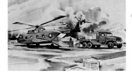
This utility version, called S-61R by Sikorsky, incorporates a rear loading cargo ramp for rapid loading of wheeled vehicles, cargo, and troops.
