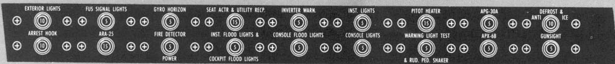
RIGHT-HAND FORWARD CONSOLE CIRCUIT BREAKER PANEL
