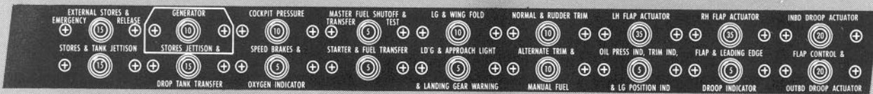
LEFT-HAND FORWARD CONSOLE CIRCUIT BREAKER PANEL
