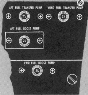
LEFT-HAND REAR CONSOLE CIRCUIT-BREAKER PANEL
