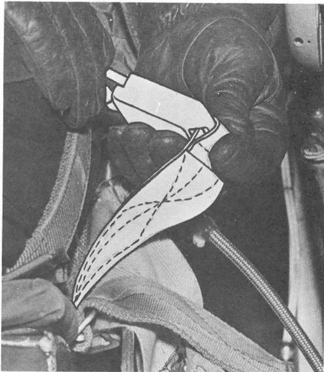
3 SURVIVAL PACK TO LOWER LEFT PARACHUTE HARNESS - ATTACH.
