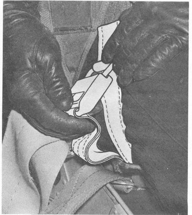
2 SURVIVAL PACK TO LOWER RIGHT PARACHUTE HARNESS - ATTACH.
