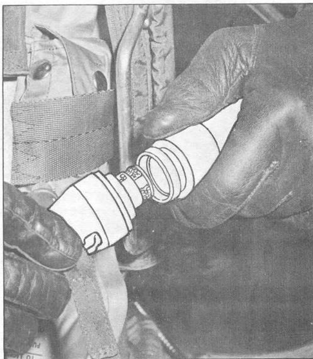
11 OXYGEN MASK HOSE - CONNECT TO SEAT OXYGEN HOSE.
