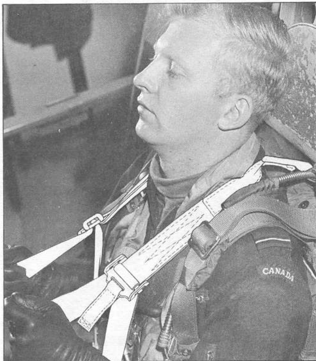
9 SHOULDER HARNESS - ADJUST UNTIL YOKE TOUCHES BACK OF NECK.
