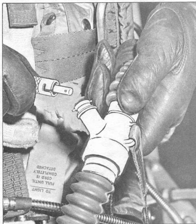
12 BAIL-OUT BOTTLE OXYGEN HOSE - ROUTE UNDER RIGHT SHOULDER HARNESS STRAP AND CONNECT TO MC-3A CONNECTOR.
