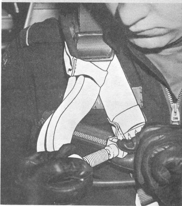
1 SURVIVAL PACK LANYARD - ATTACH TO PARACHUTE HARNESS OR LIFE JACKET (IF WORN).
