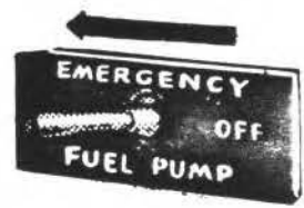
14 EMERGENCY FUEL PUMP ON
