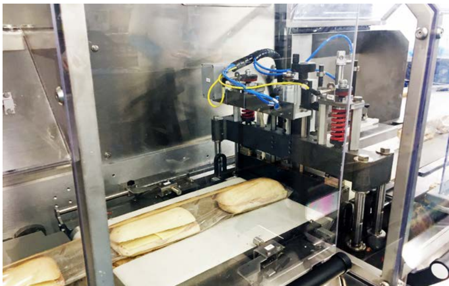
The Delta 3000 uses three rollers for making the fin seal, rather than two as is the case with most entry level flow wrappers which makes for extremely consistent sealing performance.
