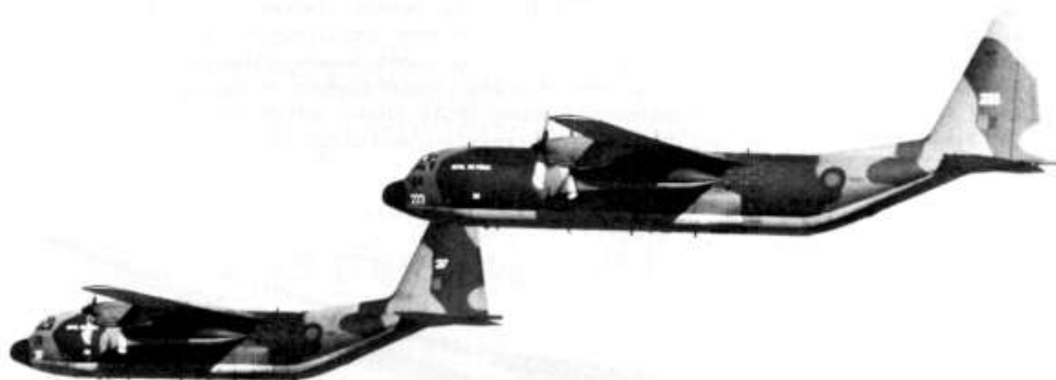
The RAF's airlift capability is to be increased by some 12 per cent by modification of 30 Hercules C Mk 1s to C Mk 3 standard, with 15-ft (4.57-m) fuselage extension. The first stretched aircraft is seen here (right) in company with a standard C Mk 1.
