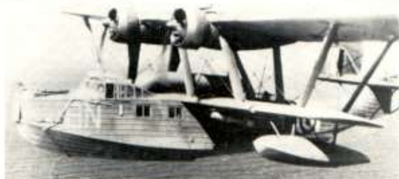
(Above) A Saro London II of No 240 Squadron, with long-range saddle tank and underwing bombs, as in service for coastal patrol when the war started.
