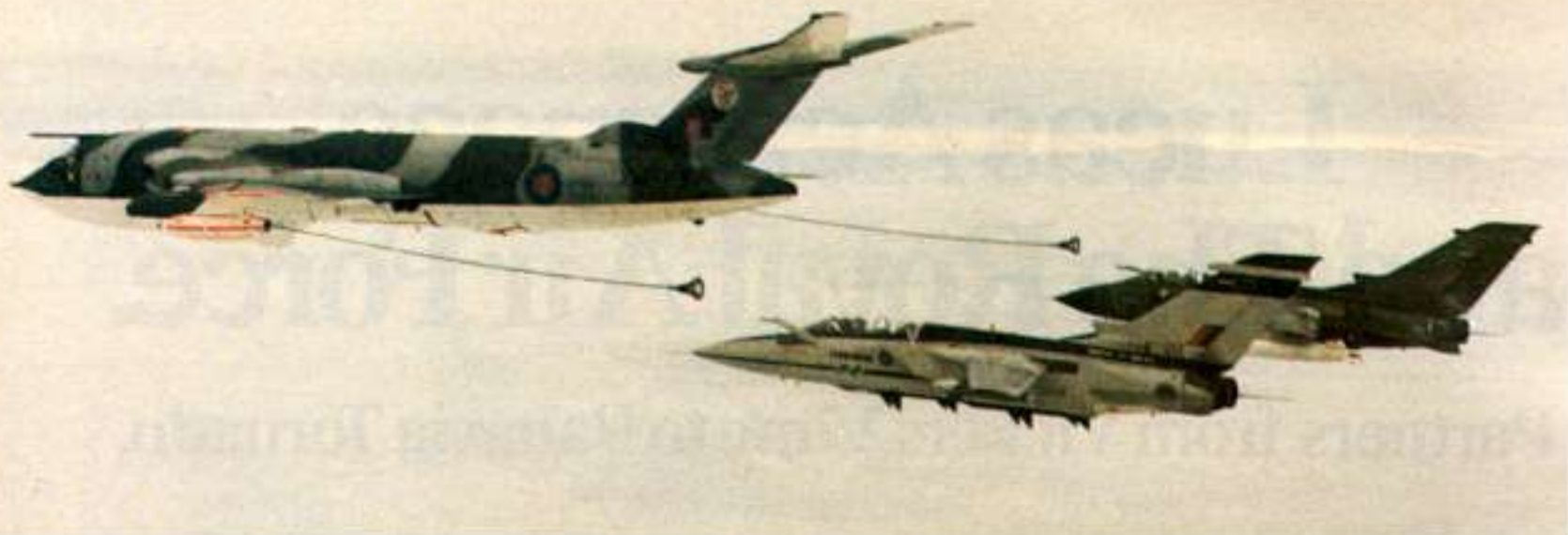
Air-to-air refuelling plays a vital rôle in RAF planning, especially in respect of the air defence of the UK. The only tanker currently in service is the Victor K Mk 2, an example of which is seen here refuelling the first prototype Tornado F Mk 2 and the last of the pre-production batch of Tornado GR Mk 1s. Starting in 1982, the RAF will receive five VC10K Mk 2s and four VC10K Mk 3s to form a third AAR squadron.
