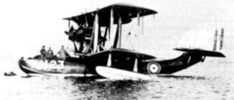
The first flying boat of post-war design to enter RAF service was the Supermarine Southampton, one of R J Mitchell's first military aircraft designs. About 20 Southamptons had wooden hulls (below) but most were converted to metal-hulled Mk IIs (above) and about 50 more were built as such.
