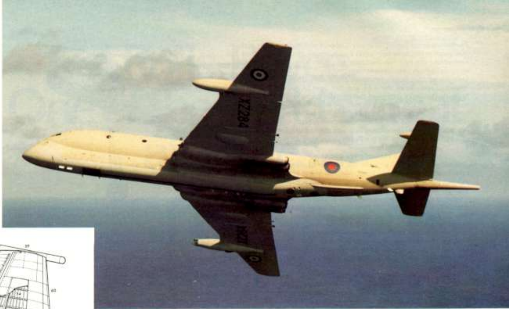
While 11 of the original RAF fleet of 46 Nimrods undergo conversion to AEW Mk 3 standard as depicted in the cutaway drawing here, the balance of the maritime reconnaissance aircraft are in process of being updated to Nimrod MR Mk 2s (above) featuring a new equipment fit and new colours.
