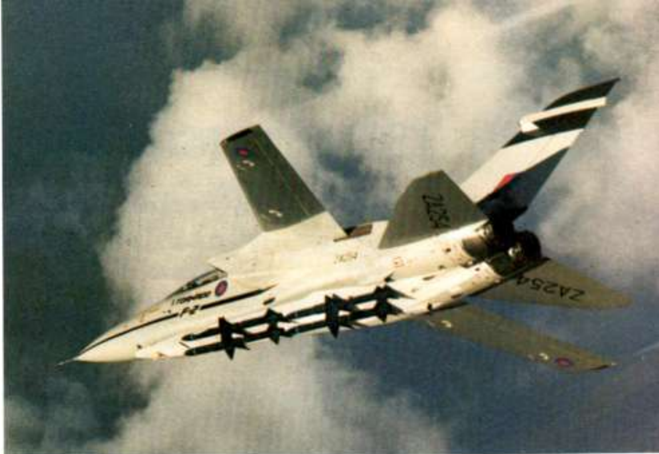
In addition to the Tornado GR Mk 1s (see previous page), the RAF is to receive 165 of the F Mk 2 air defence variant, the prototype of which is seen above. As the photograph and cutaway drawing show, the Tornado F Mk 2 has a longer fuselage, longer nose radome, revised weapons system and other changes.
