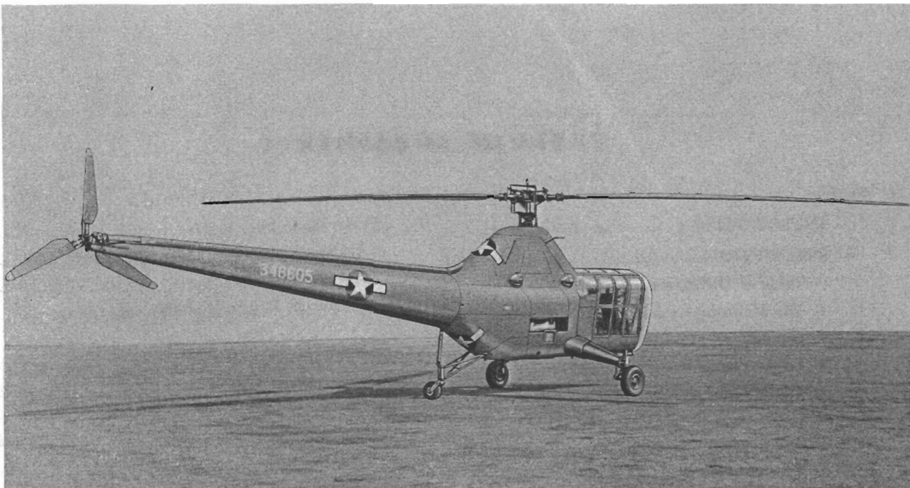
Figure 1—Three-quarter Rear View, R-5A and R-5E (Model R-5D has wider cabin and a nose wheel)
