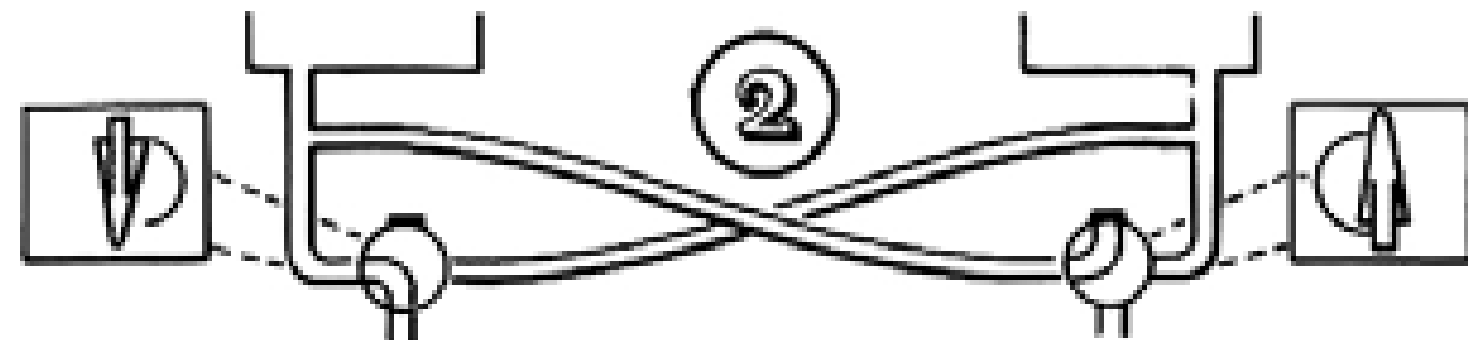
LEFT ENGINE OPERATION - Left tank to left engine, right engine off.
