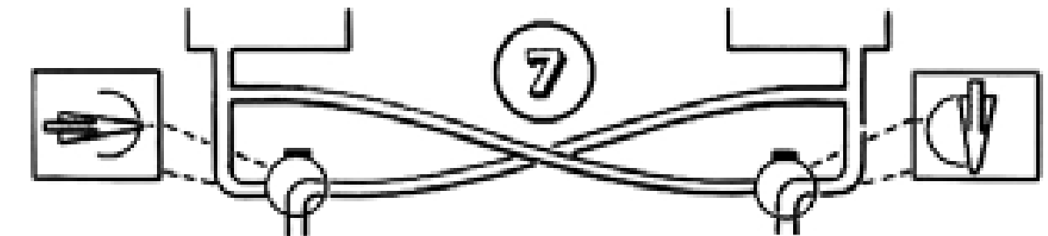
BOTH ENGINES FROM RIGHT TANK
