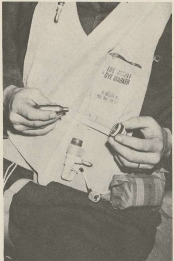
Check CO 2 inflator before flight. See that the cartridge seal is not punctured. The puncturing arm should be in a vertical position, and safetied with light wire. The cartridge goes in with small end down. Screw the cap down tight when you replace it.
