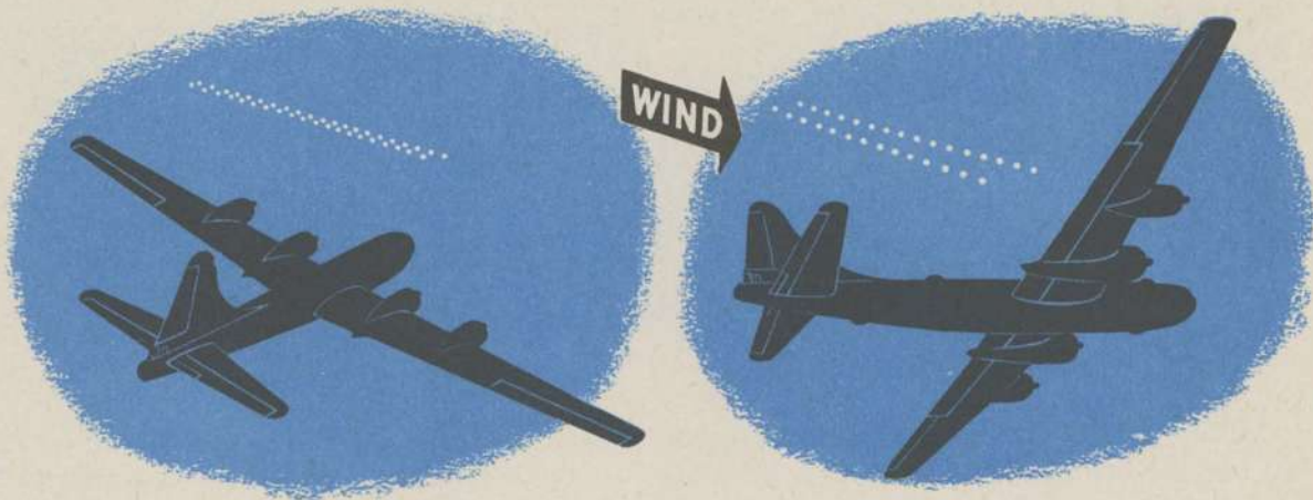
TURN INTO APPROACH FROM BASE LEG WHEN RUNWAY LIGHTS SEPARATE INTO TWO ROWS
