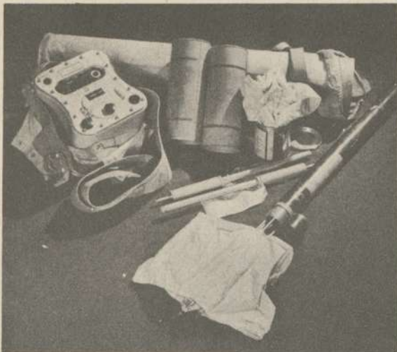
Emergency radio. Accessories include: balloon and kite for raising antenna, hydrogen generators for inflating balloon, signal lamp, extra roll of antenna wire, and an instruction book.
