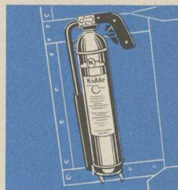
One CO 2 type fire extinguisher is located in the aft pressurized compartment
