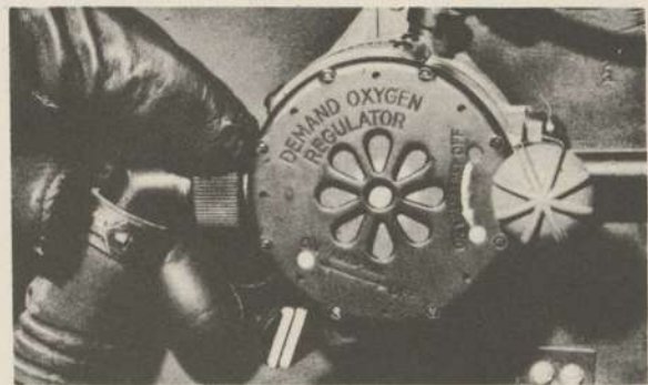
Check tightness of knurled collar.
