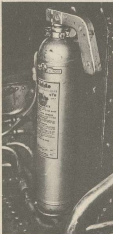
CO 2 type extinguisher located on inboard side of flight engineer's control board.
