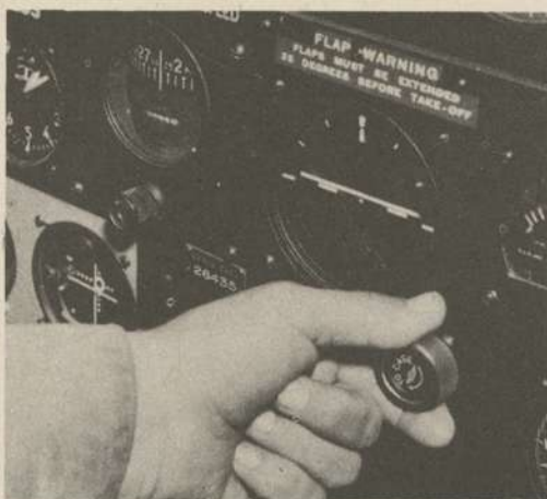
CHECK GYRO INSTRUMENTS
