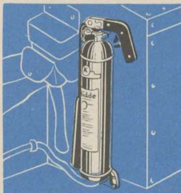
One CO 2 type fire extinguisher is located on the side of engineer's stand
