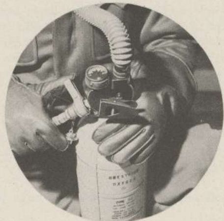
Recharging the D-2 walk-around bottle.
