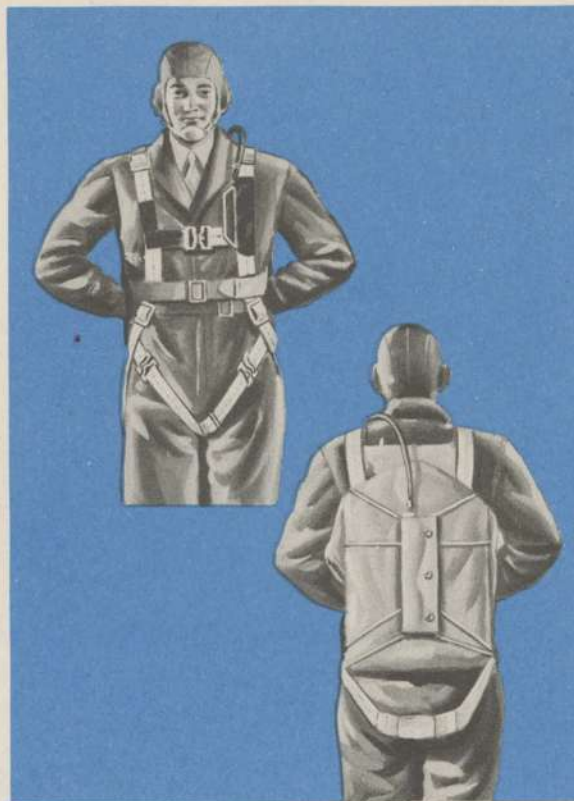
Back-type parachute. Note: If not wearing life vest, tie first-aid packet to parachute harness. When you have the bailout bottle on the right strap, put the first-aid packet on the left strap.
