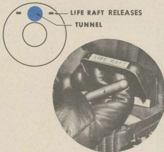
There are two raft release handles. Pull both handles to release and inflate both rafts.
