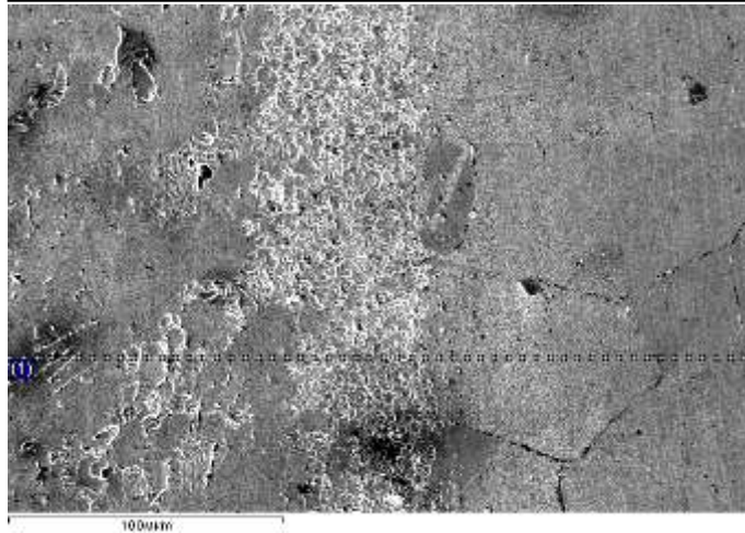
Microstructure and distribution of elements in RBW joint after heat treatment
