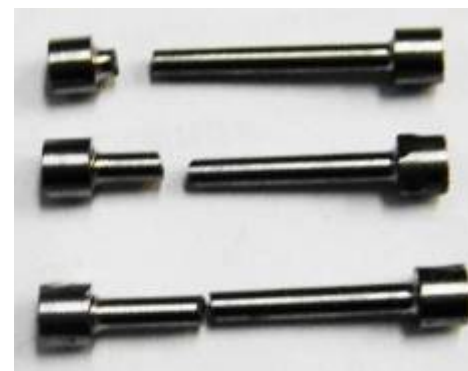
Samples of joints after rupture testing (fracture runs through BM)
