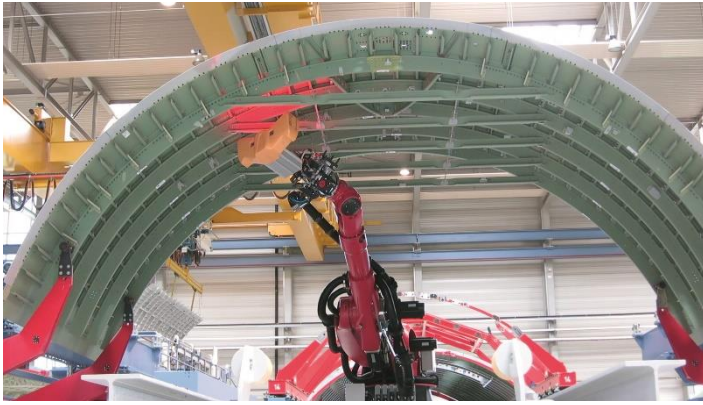
Fig.2.8 Fuselage section assembly inspection system
