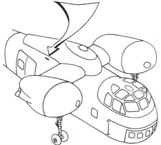
Figure 4-3. Heater Fire Detector Panel
