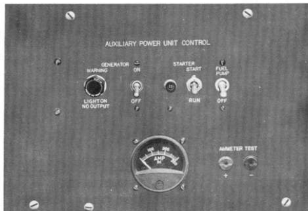
Figure 4-13. Auxiliary Power Unit Control Box
