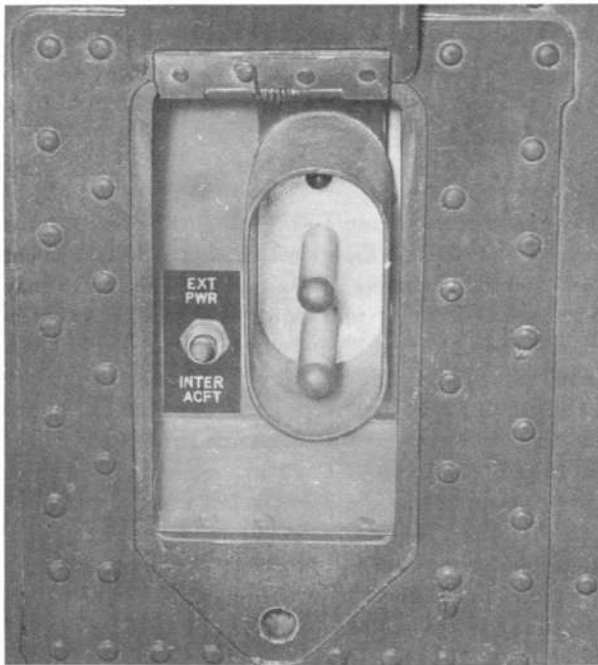
Figure 1-23. External Power Receptacle and Switch
