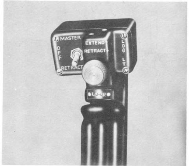
Figure 4-11. Landing Light Switches
