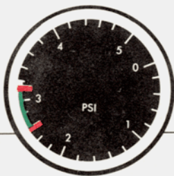
UTILITY SYSTEM HYDRAULIC PRESSURE
