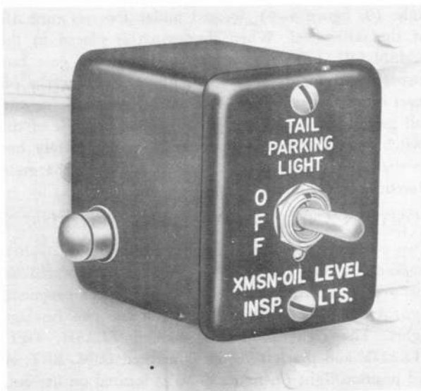
Figure 4-10. Parking and Gear Box Inspection Light Switch
