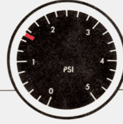
EMERGENCY SYSTEM HYDRAULIC PRESSURE
