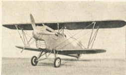
KAWASAKI ARMY 8-95 single-seat fighter, one 600 h.p. Kawasaki motor. Span, 35 ft.; max. speed, 250 m.p.h. Armament, three fixed machine guns.
