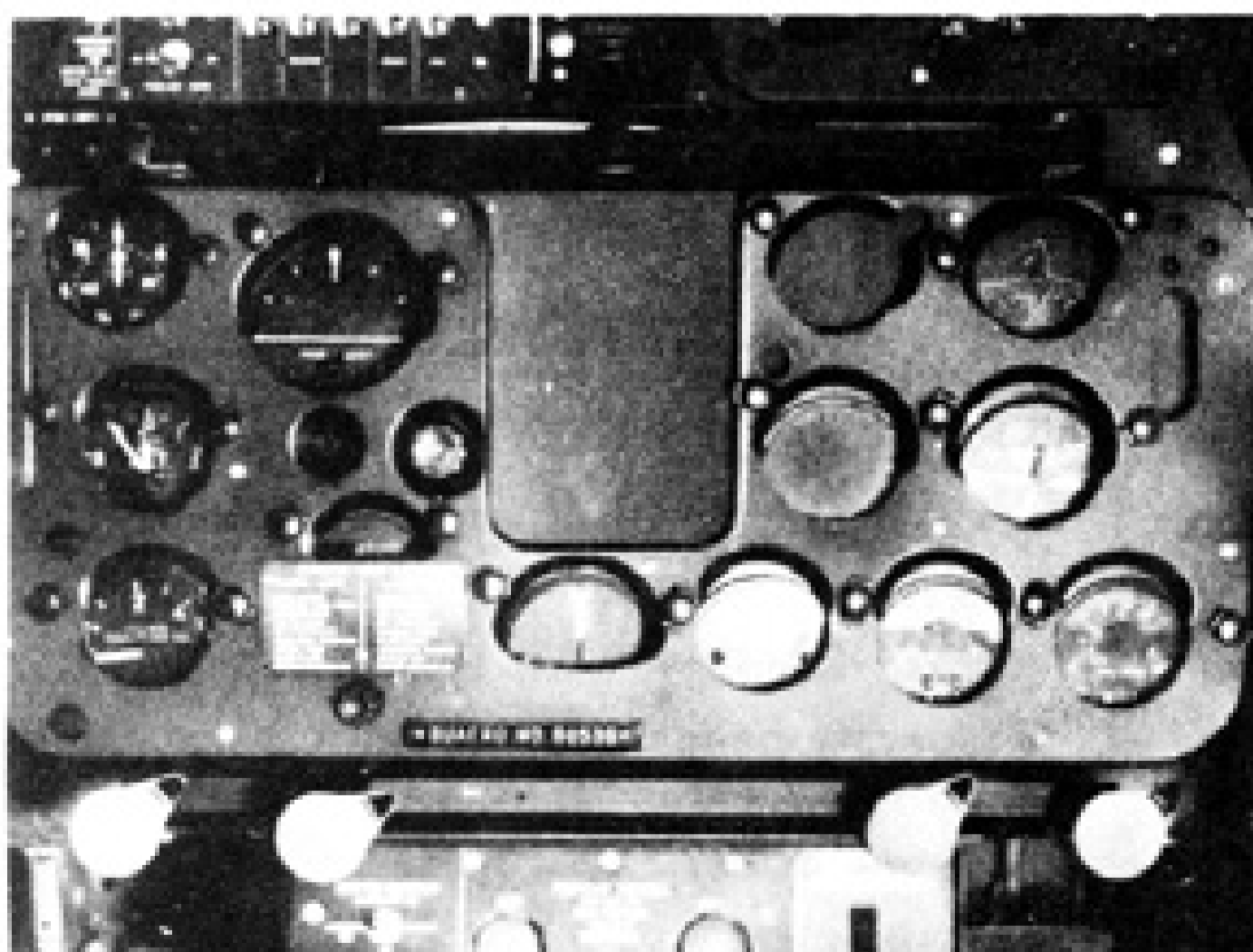
Figure 43—Gun Charging Controls
