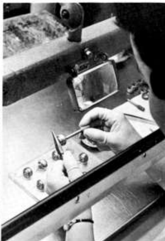
HAWK GYROS and accelerometers are assembled in a clean room at Raytheon's Andover plant. Production techniques are conventional; accent is on quality control and careful inspection following every few steps of assembly.
