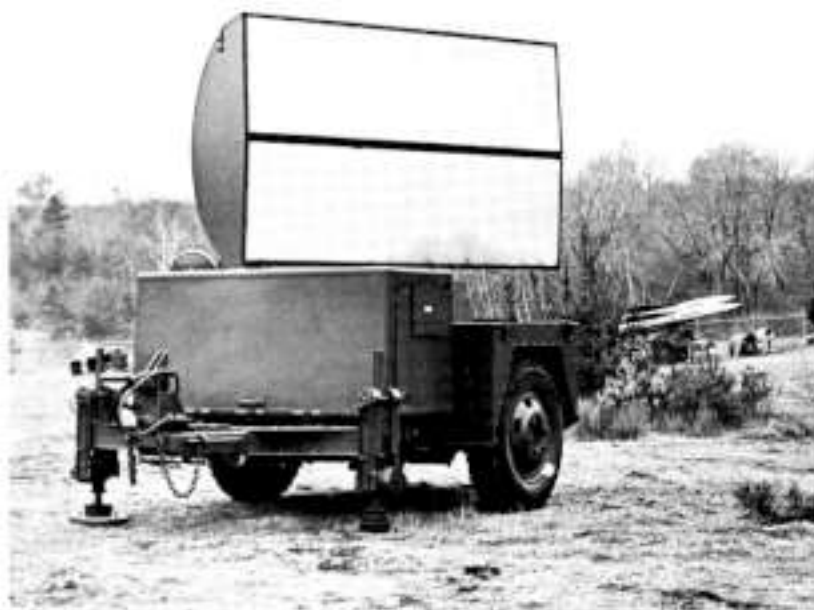
HAWK battery equipment includes AN/MPQ-34 cw acquisition radar (above) and AN/MPQ-33 cw illuminator radar (upper right). Three Hawk missiles, ready for transport as a unit to launcher, are mounted on pallet attached to wheeled trailer (below). Crane beam has been added to loader (lower right).
