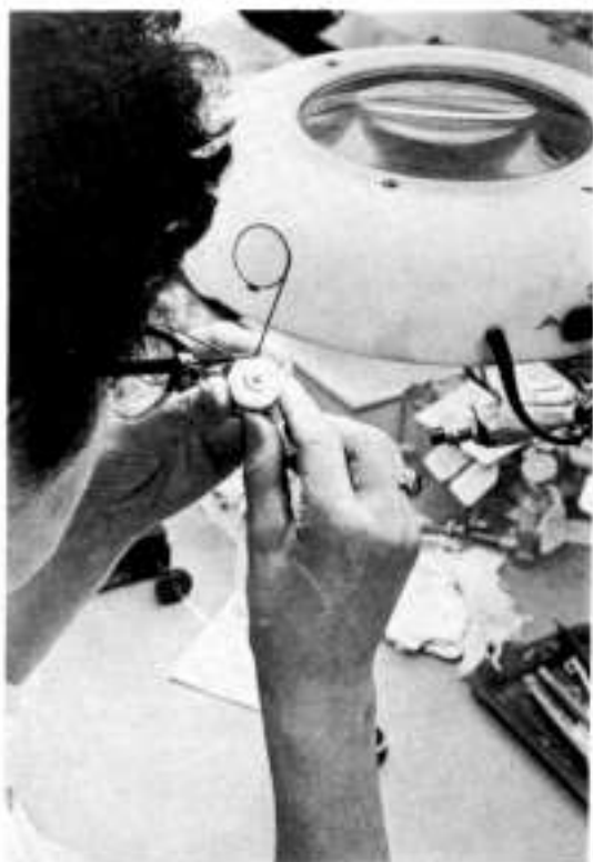
HAWK GYROS and accelerometers are assembled in a clean room at Raytheon's Andover plant. Production techniques are conventional; accent is on quality control and careful inspection following every few steps of assembly.
