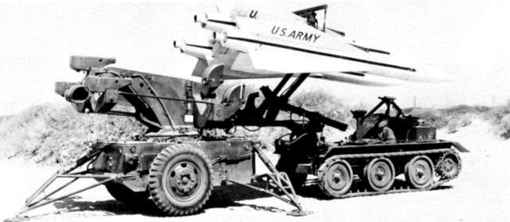
THREE HAWK MISSILES are carried to launcher and loaded, ready for firing, by tracked loader/transporter vehicle.
