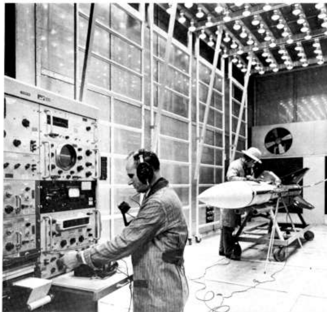
ENVIRONMENTAL TEST of Hawk missile airframe is one of rigorous set of checks made on system components during manufacture.
