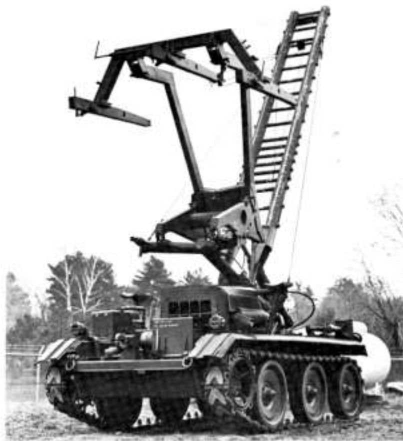
HAWK battery equipment includes AN/MPQ-34 cw acquisition radar (above) and AN/MPQ-33 cw illuminator radar (upper right). Three Hawk missiles, ready for transport as a unit to launcher, are mounted on pallet attached to wheeled trailer (below). Crane beam has been added to loader (lower right).
