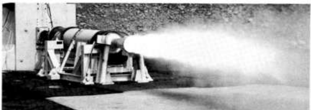
AEROJET-GENERAL solid-propellant rocket engine for Hawk missile fires at two thrust levels: boost (above) and sustaining for cruise (below).
