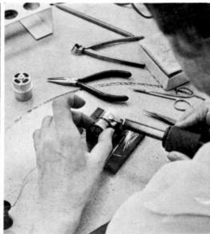
HAWK GYROS and accelerometers are assembled in a clean room at Raytheon's Andover plant. Production techniques are conventional; accent is on quality control and careful inspection following every few steps of assembly.
