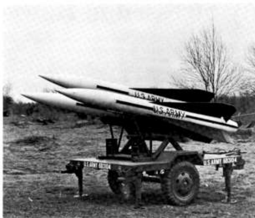
HAWK battery equipment includes AN/MPQ-34 cw acquisition radar (above) and AN/MPQ-33 cw illuminator radar (upper right). Three Hawk missiles, ready for transport as a unit to launcher, are mounted on pallet attached to wheeled trailer (below). Crane beam has been added to loader (lower right).
