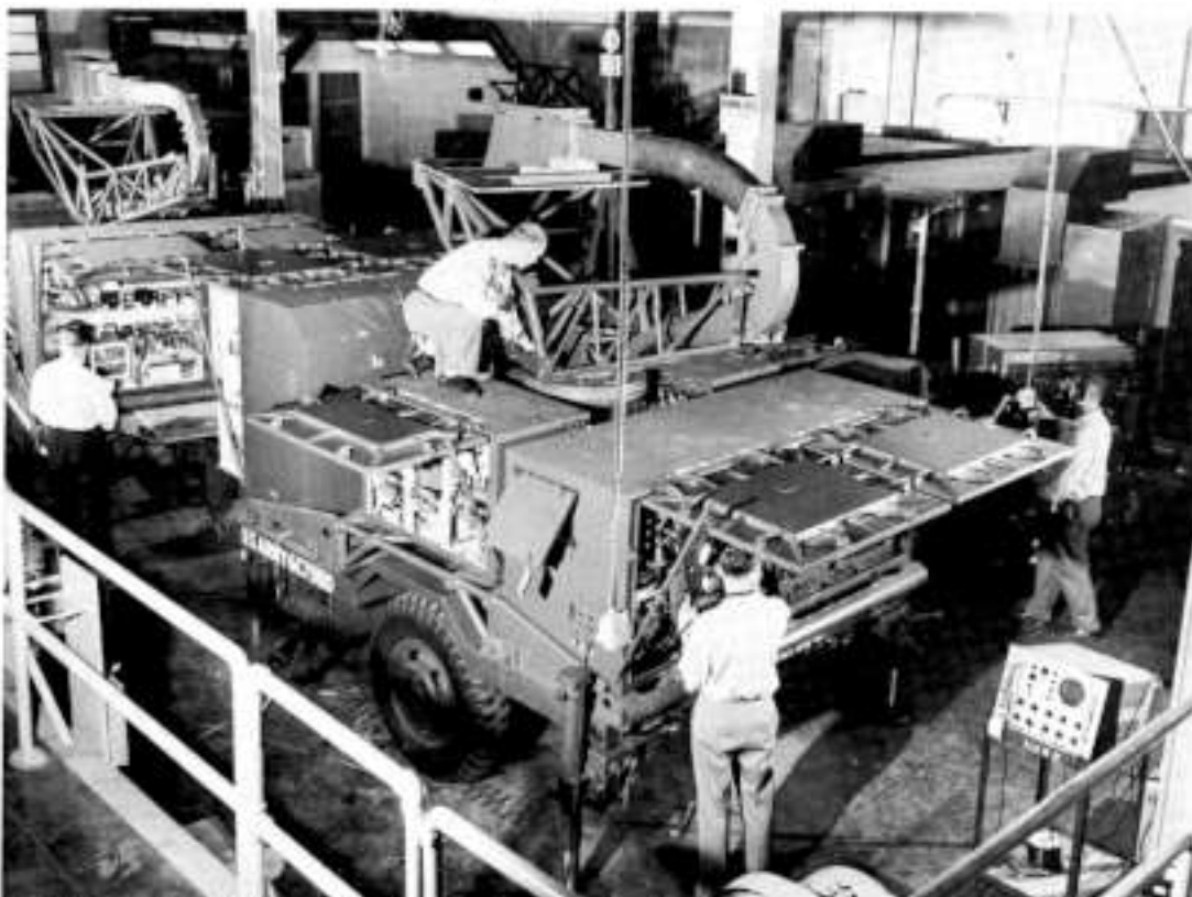
AN/MPQ-35 pulse acquisition radar for Hawk missile system gets electronic check during final assembly at Raytheon's Waltham plant. Dummy load replaces paraboloid antenna on top of palletized radar assembly. Unit is wheeled for over-the-road towing, breaks into two sections for helicopter transport.
