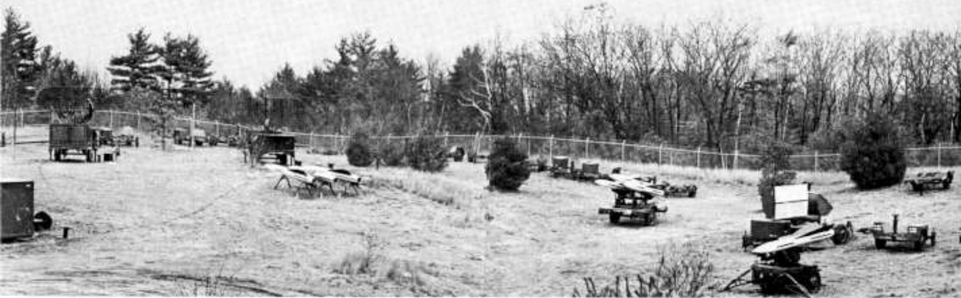
testing of missile system. Engineer enters battery control central (left); cw acquisition radar is in left foreground.
