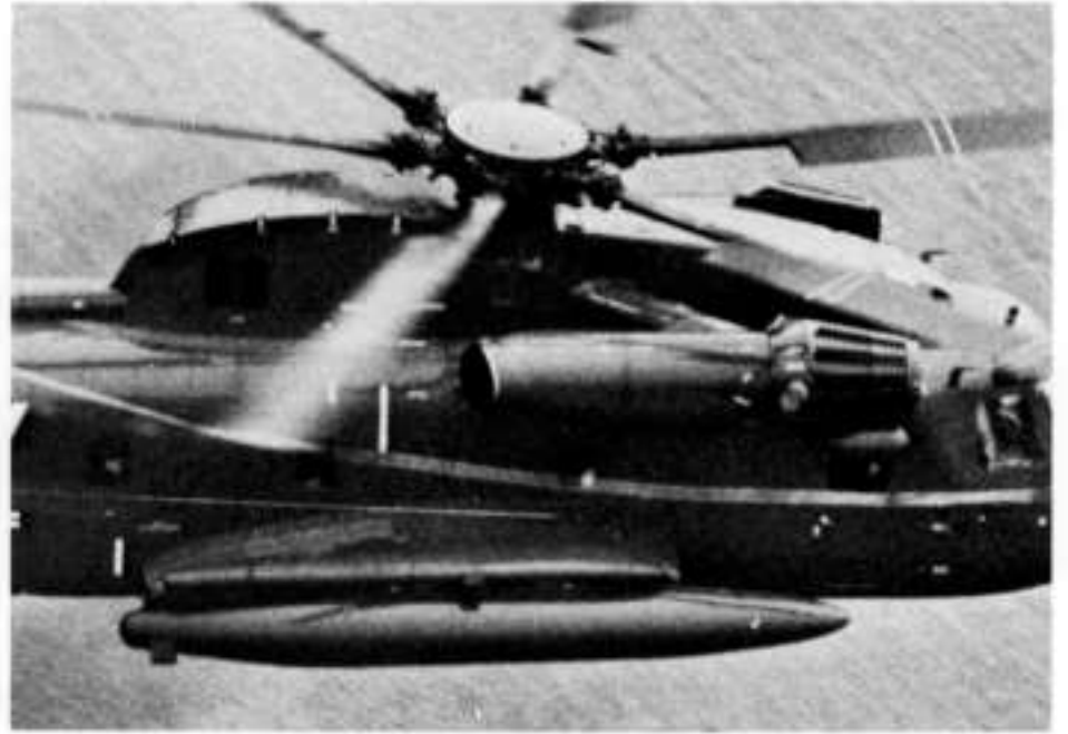
RH-53D with 2460 liters (650 Gal.) Auxiliary Fuel Tank
